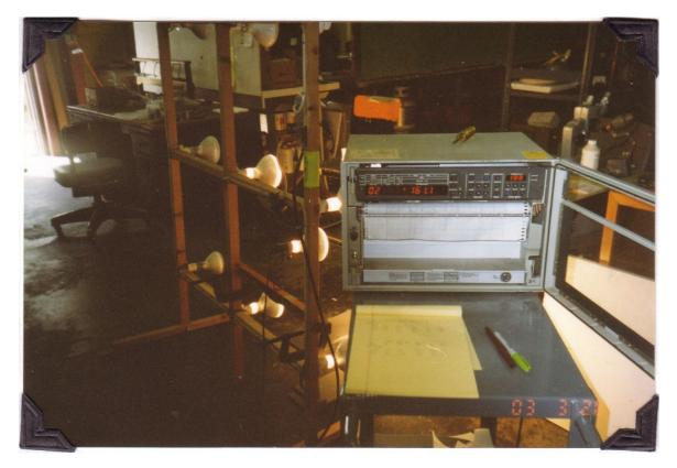
Photograph of the millivolt recorder and solar lamp array
