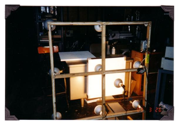
Photograph of the solar lamp array and Insuladd painted wall panel
